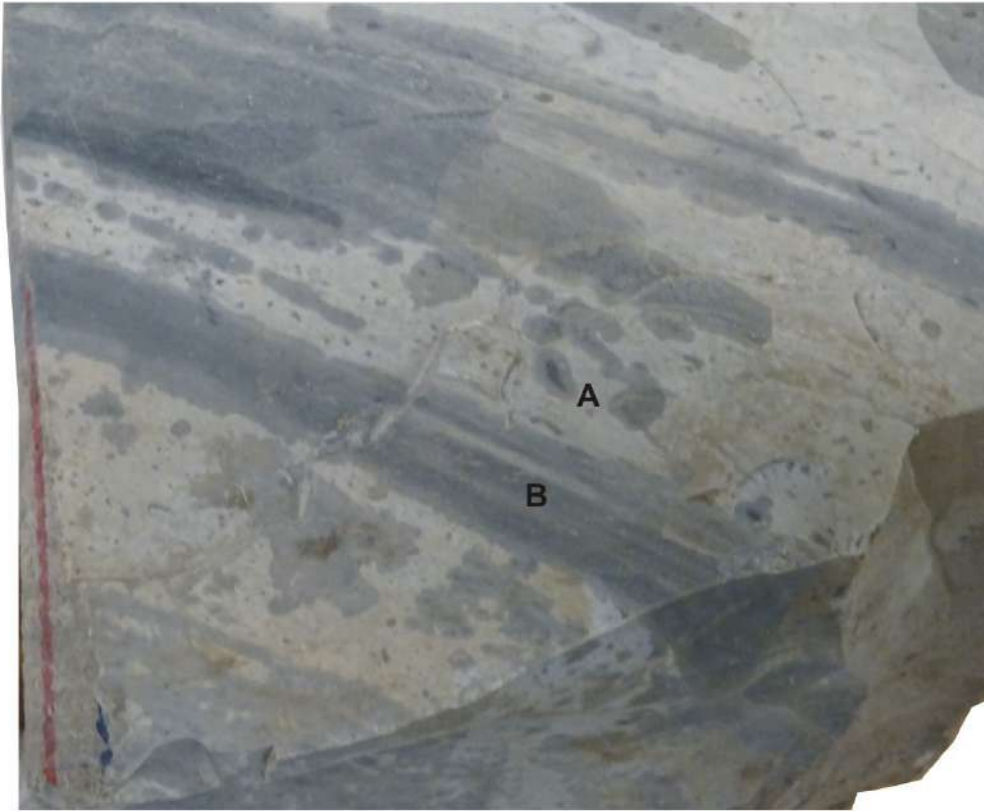
Fig. 11 - A massive flint bed from the North Sea Dan field, which can be followed between several boreholes (Fig x). The flint is grey and white with geyish burrows (A) and layering (B). The flint vary between non-bioturbated and bioturbated layers. The flint is a porcelanite. ME-1 borehole 7213 ft (2383,75 m), Maastrichtian limestone of the Tor Formationen. 20 cm wide.
