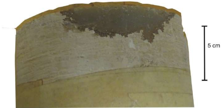
Fig. 9 - The surface of the flint is very irregular which may reflect the solution of the chalk and the precipitation of the silica. Similar pattern can be observed on the surface of erratic flint blocks in Quaternary tills. Dan Field wellbore ME-1 at 7167.6 ft.
