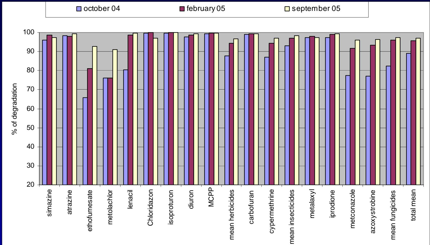
75 % of biofilters present a degradation > 91% (minimum = metolachlor)
