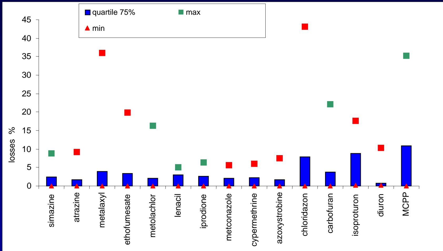
75 % of biofilters have an efficiency > 90 % for all the molecules analysed
