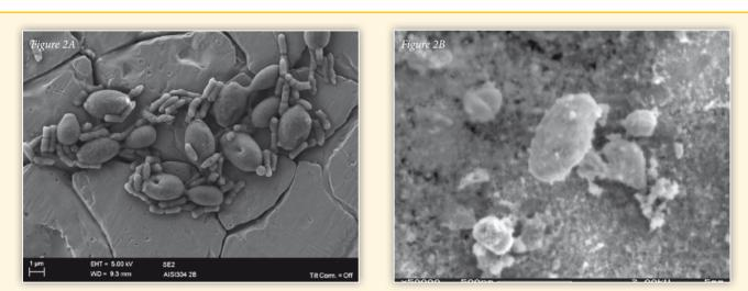
Figure 2. Microbes on stainless steel surface A) in the laboratory and B) on a sample coupon from a one-year process study.
