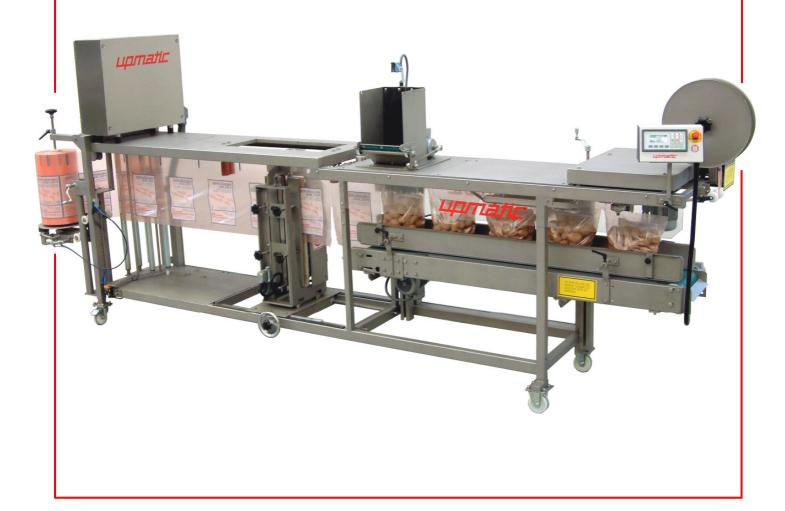
Upmatic 2000E = fully automatic filling and sealing machine for polyethylene bags ranging from 0,5 kgs to 10 kgs filled weight. Suitable for all bulk and granular products of the food and non-food industries.
