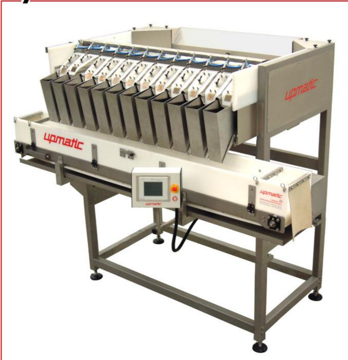
Upmatic Type 2212 = computer controlled proportioning component weighing machine for fine and coarse products in the food and non-food industries. The weighing range covers, dependent on product, all weight classes from 100g to 5000g (higher weights by double dumps).
