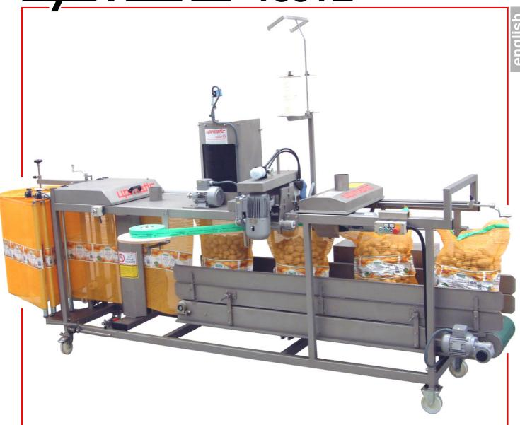
Upmatic 1351E = fully automatic filling and sealing machine for split-film woven polyethylene bags ranging from 2,5 kg to 25 kgs filled weight. According to the choice of packing material, it is suitable for all bulk and granular products of the food and non-food industries.
