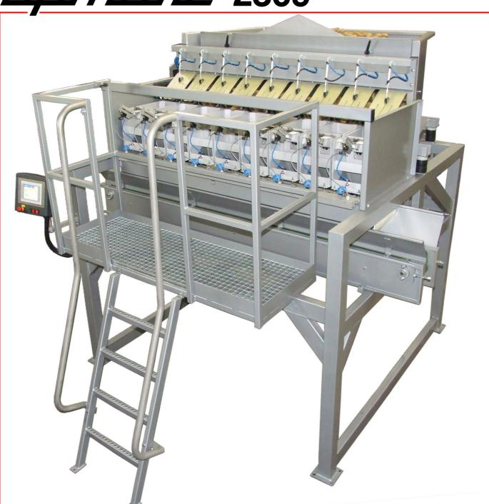
Typ 2309 = computer-controlled, Upmatic proportioning component weighing machine for fine and coarse products in the food and nonfood-industries. The weighing range covers all weight classes between 1 and 25 kgs - weighing without losses.
