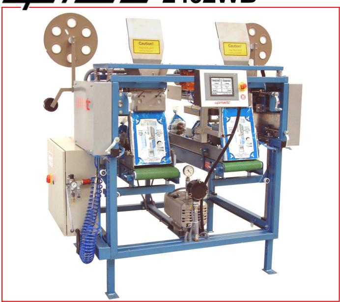
Upmatic 2402WB = fully automatic filling and closing machine for polyethylene bags from 1 up to 10 kgs. Suitable for all bulk and granular products of the food and non-food industries
