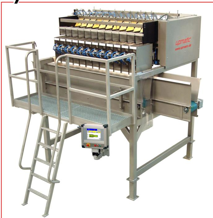
Upmatic 2112KE = computer-controlled, proportioning component weighing machine for fine and coarse products in the food and non-food-industries. The weighing range covers all weight classes between 0,5 and 25 kgs – weighing without losses.
