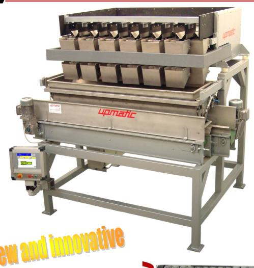
On demand, the pre-dosing weighing buckets are swiveable without use of any working tools.
