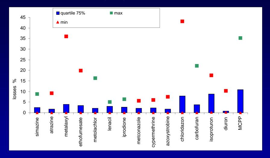
75 % of biofilters have an efficiency > 90 % for all the molecules analysed > 96 % excepted chloridazon, isoproturon and MCPP
