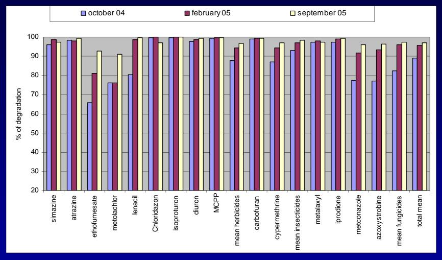
75 % of biofilters present a degradation > 91% (minimum = metolaclor)
