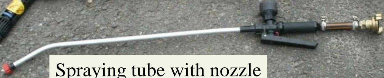
Spraying tube with nozzle
