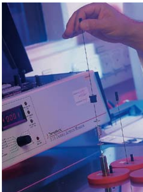
Thermal Activity Monitor for accurate measurement of the decomposition rate of organic peroxides
