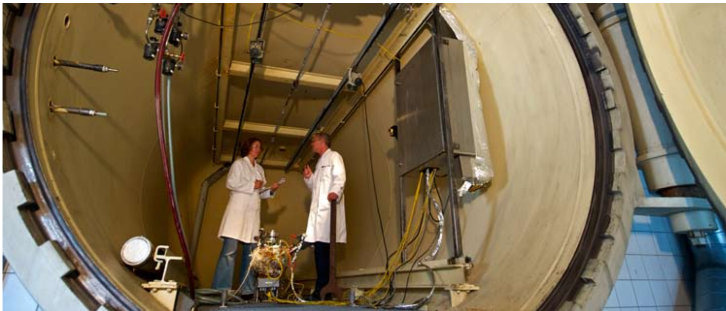
55 m 3 total containment tank for large-scale safety testing in Deventer, the Netherlands
